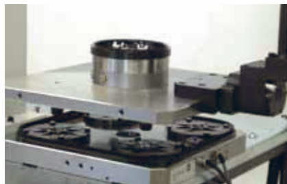
Universal combination of EROWA clamping systems with automatic handling.
