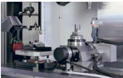
Flexible and automatic loading of a machine tool with an EROWA handling unit. The ratio of productive hours is considerably increased.
