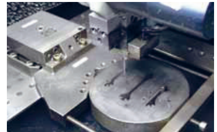
Special accommodation for cylindrical parts. Fitted to the pendulum holder, workpieces can be adjusted in three axes.
