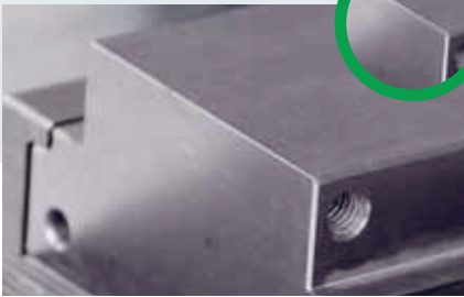
Smooth clamping surface
