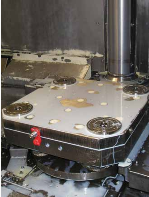
The module interior is completely sealed. As a result, the system is optimally protected against liquids and dirt.
