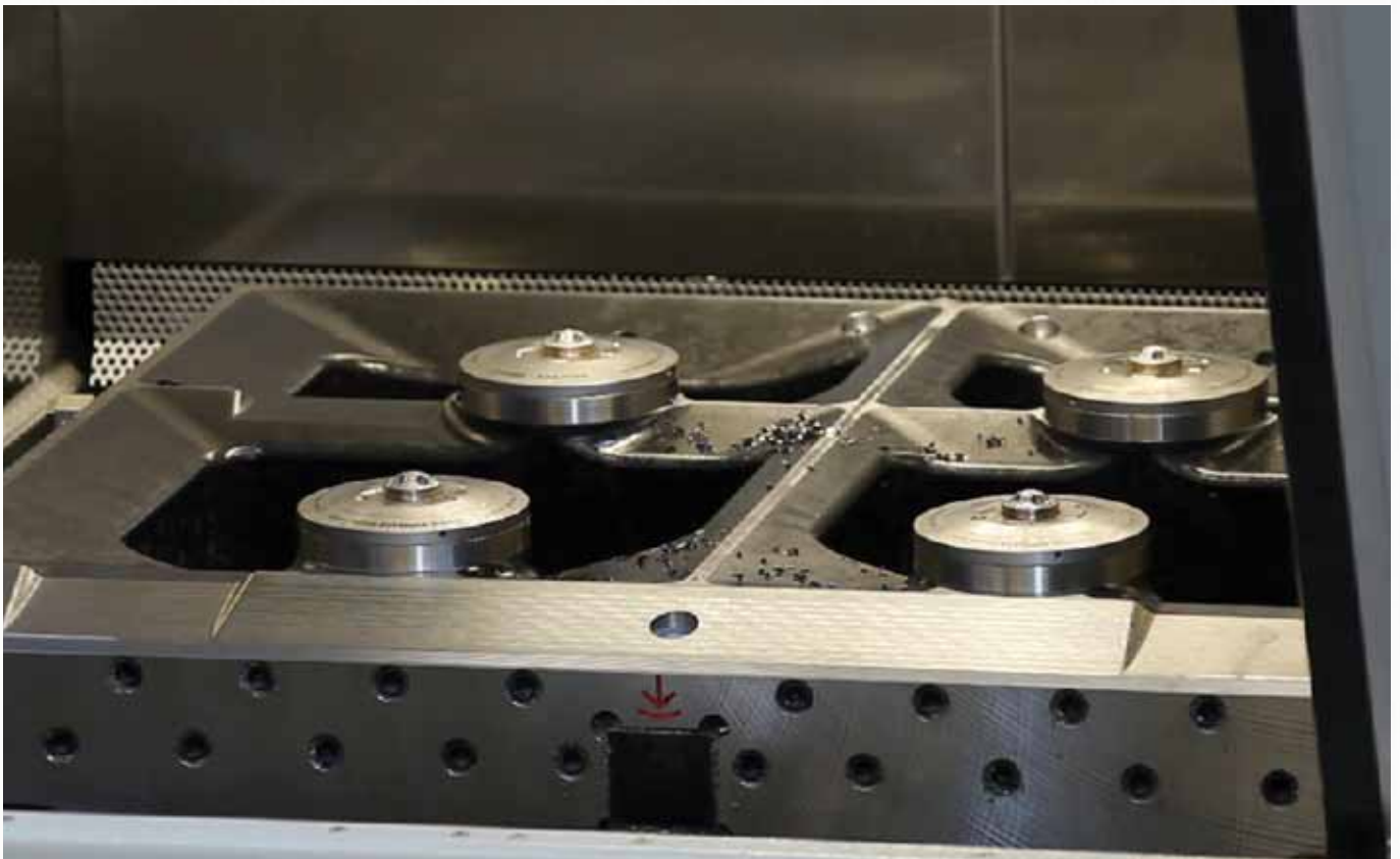
„Turbine“ high-end clamping module (order no. 420919) in use in a fully automated production process with robot loading.
