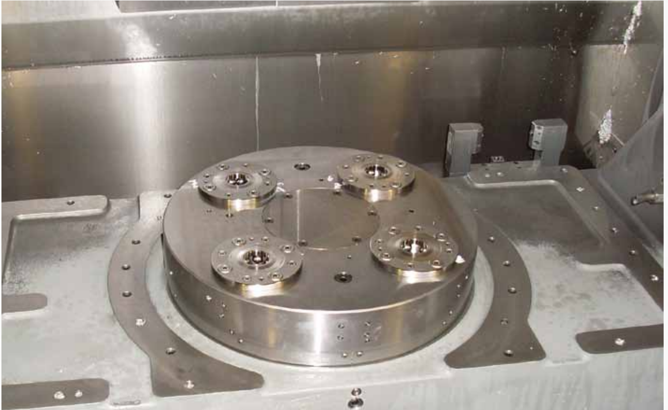
Automation solution (order no. 427161) with lock and support control as well as nipple sensing in use in a fully automated production process with robot loading.
